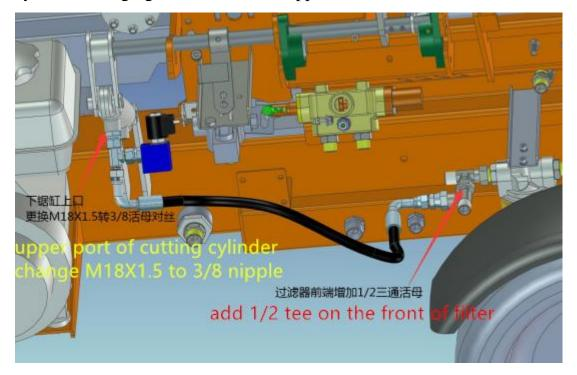
Add 1/2 tee connector to tee connector on the front of filter
