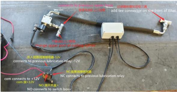
Every time chainsaw plate/bar goes back to original position, it will activate the solenoid valve for about 1s by inching switch, then close.
